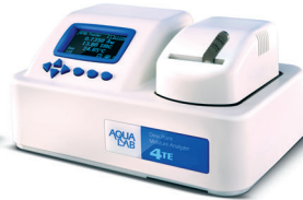
4TE Water Activity Meter. Temperature Control (Between 15-50°C).
